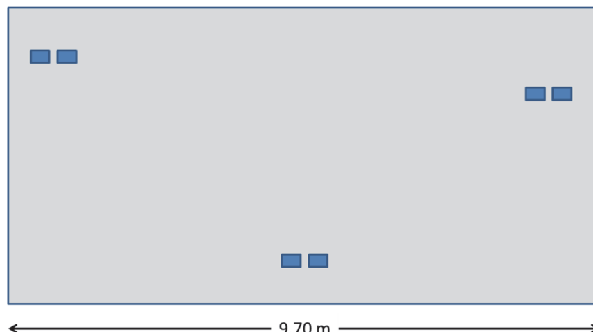
Figure 1 – Graphic shows desired layout of specimen collection sites on a cover top. Specimen collection sites are approximate and should be located to avoid seams or welds. Each specimen of the pair should be uniquely marked.
