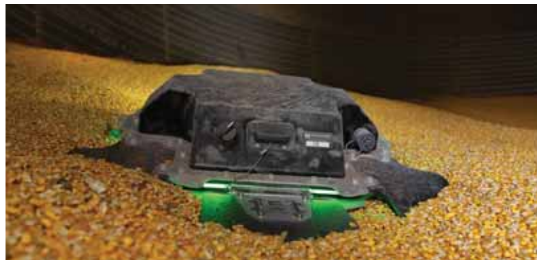
The Grain Weevil Robotics Platform removes the need for anyone to physically enter a grain bin.
