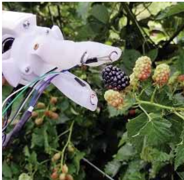
Researchers at Mississippi State University, in collaboration with Georgia Tech and the University of Arkansas, have developed a robotic blackberry picker (photo by Anthony Gunderman, Georgia Tech and University of Arkansas System Division of Agriculture).
