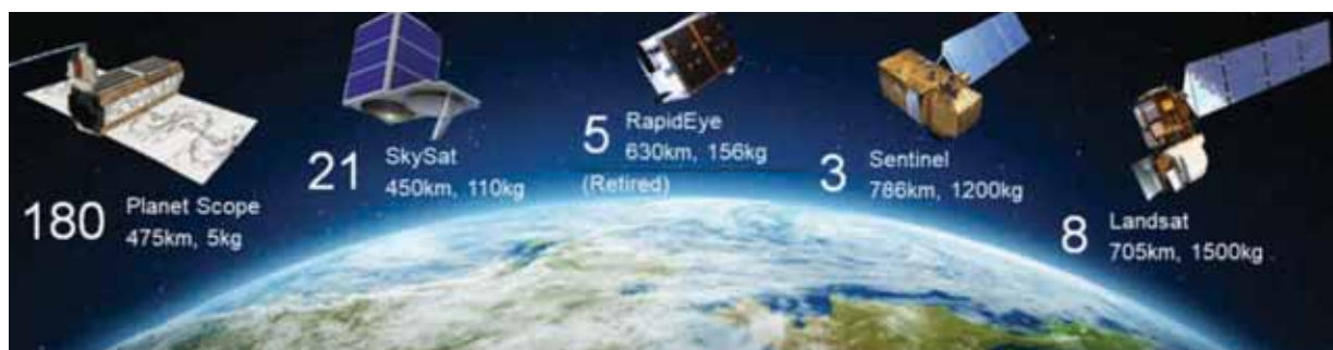
Examples of satellites from commercial (Planet Scope, SkySat, and RapidEye) and public (Sentinel and Landsat) sources, showing the number of satellites, altitude, and weight. They all operate in Sun-synchronous orbit (SSO).
