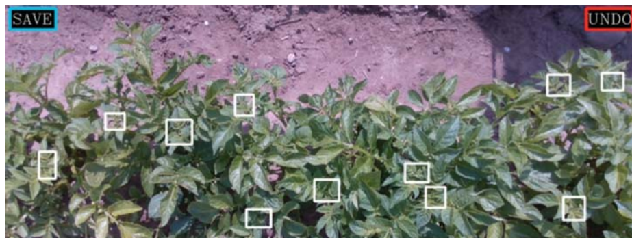
Potato stem identification and counting using computer vision AI.
