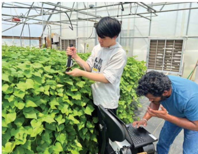
Collecting hyperspectral reflectance data for phenotyping.
