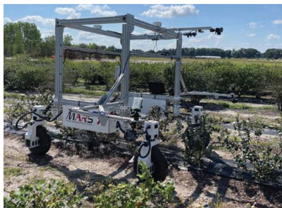
The customized mobile robot, called MARS-X, performs real-time crop phenotyping. It carries a multi-view imaging system, and a lightweight graph neural network model runs in real-time on its embedded computer.
