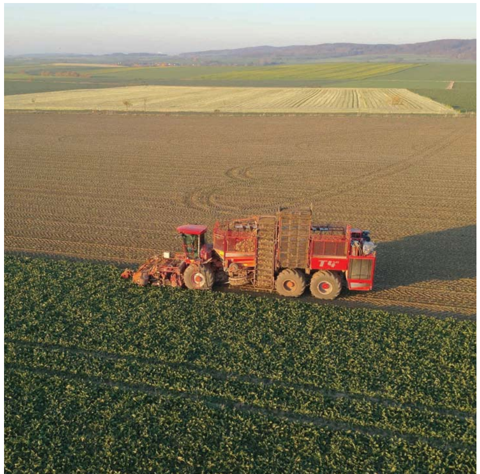
A self-propelled sugar beet harvester at work in a European field.
