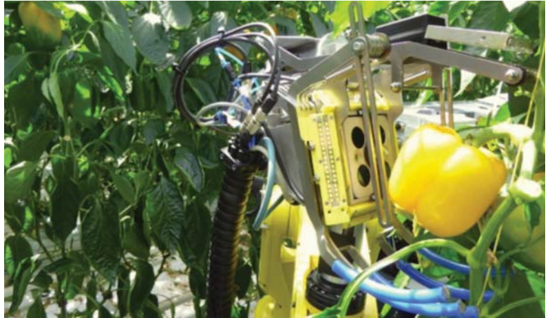
The EU-SWEEPER selective harvester for sweet peppers (photo courtesy Wageningen University and Research).
