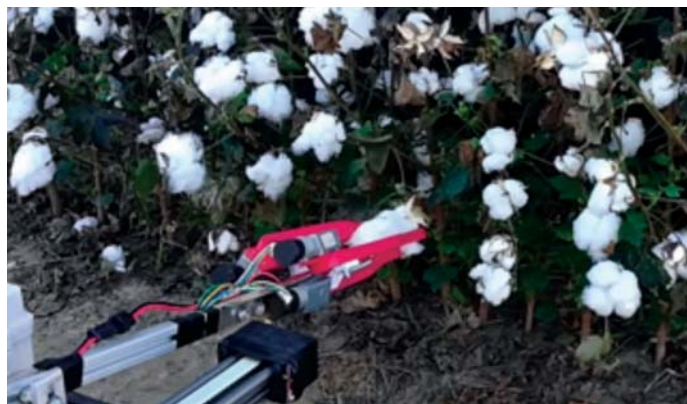
Robotic harvesting of cotton bolls.
