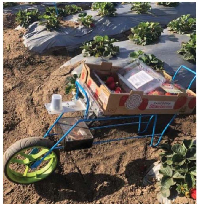
Each worker has a customized cart, called iCarrito, that transmits its location and its tray weight. When the tray is full, a FRAIL-bot arrives to carry it to the collection station (photo courtesy of Stavros Vougioukas/UC Davis).
