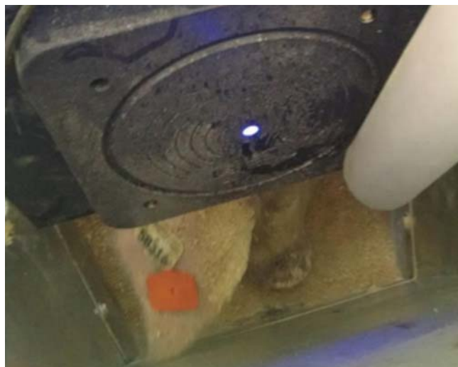
Figure 5. An RFID reader above a sow’s head during feeding. The sow’s time at the feeder is logged by the reader.
