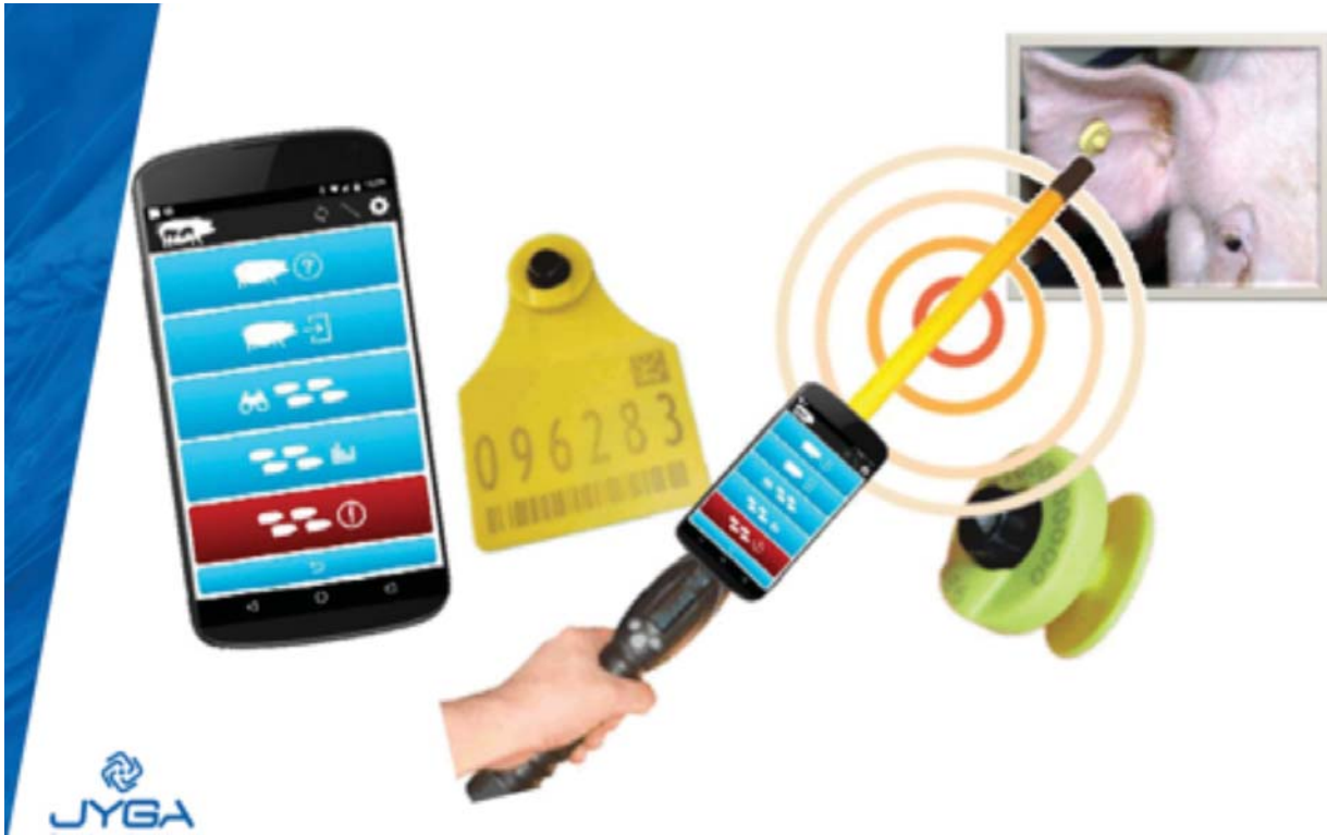
Figure 6. A wireless handheld reader can read RFID tags similar to a stationary reader.
