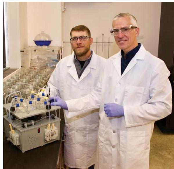
ASABE member Jacek Koziel (right) and research collaborator Devin Maurer, with a prototype of their new tool that can dramatically speed detection of bovine tuberculosis by identifying the unique signature of the gases that different microbes emit over time.
