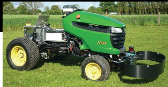
"Norman," a seeding robot designed to put seed in the ground even at field capacity (seeder to be developed this year).
