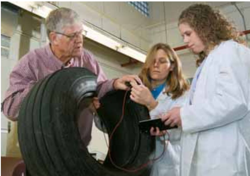
ASABE member Gary Krutz and graduate research assistants Timu Gallien and Alyssa Brune conduct research on a “smart” tire designed to sense tread damage before the tire goes flat or experiences tread loss. (Photo courtesy of Purdue University)
