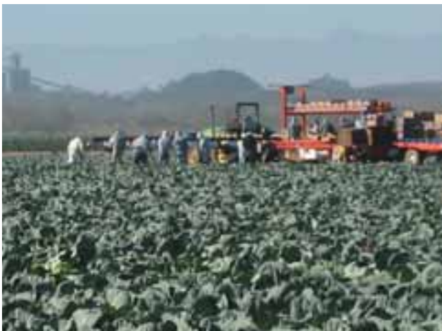
Note the driverless tractor working with a cabbage-harvesting crew of 20. Tractors may operate up to 3.2 kph (2 mph) without a driver if the throttle, brakes, and clutch pedal are remotely controlled.
