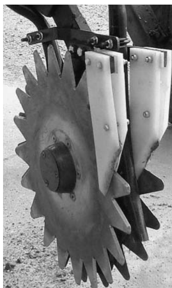
StubbleStar® no-till seeder opener showing stars and tooth cleaners.
