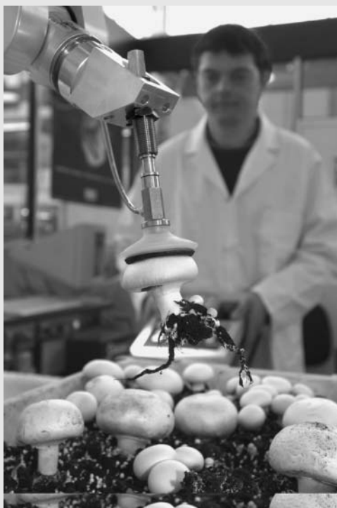
This robotic mushroom picker uses a charged coupled camera to select mushrooms that are the right size for picking. (Photo courtesy of the University of Warwick)
