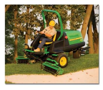
can be shifted outward to extend the cutting unit beyond the outer edge of the tire for trimming. Shifting only one cutting unit helps keep the machine's center of gravity more consistent, maintaining the machine's overall stability.
