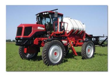
The Miller Spray-Air™ air boom system, up to 36.6 m (120 ft) wide with dual fans on the G75, may be optioned to either model. The SmartDrive® hydrostatic front-wheel assist system from Poclain® is available on the Condor G75 and features on-demand engagement and disengagement, as well as the ability to run engaged full time. To increase the productivity potential for the G40, a 4,542 L (1,200 gal) tank option has been added. Also available are a fixed axle and an auxiliary light kit.
