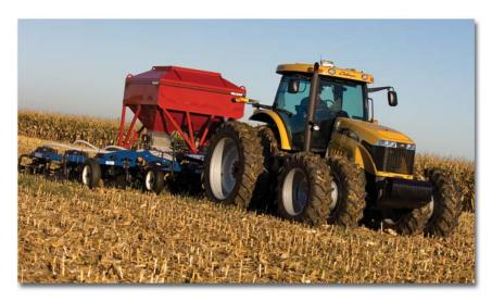
exit the exhaust into nitrogen and water with dramatic fuel savings over other technologies. The Dynamic Tractor Management System coupled with our continuously variable transmission (CVT) provides simple and efficient operation, allowing the tractor to automatically adjust to loads, to maximize fuel efficiency. The redesigned cab has 3.3 m<sup>3</sup> (116.5 ft<sup>3</sup>) of interior space, along with OptiRide cab suspension, and a new seat-mounted control console.
