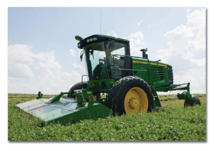
ments, and the IntelliAxle with torsional axle suspension and rear steering assist system. The windrower also boasts increased serviceability and a John Deere Tier 3 PowerTech E engine. The 400 Series windrowers are available in two configurations: a 125 hp A400, designed for auger platforms, and the 200 hp R450, designed for use with John Deere's proven rotary platforms.
