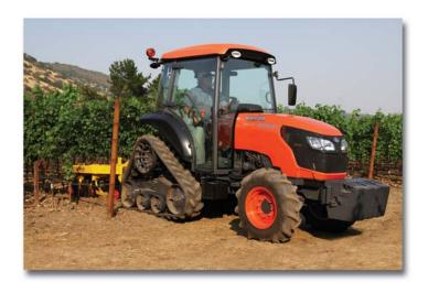
keep in contact with the ground via independently oscillating crawlers. The maintenance and process for changing crawler tracks is user friendly due to the split-type drive sprocket design with rotating pins. The Power Krawler's features build on the standard narrow tractor, with a year-round environment-controlled cab, a low overall height of 2.3 m (92 in.), and the power of Kubota's M-series engine, which increases the performance and maneuverability in narrow-row applications.
