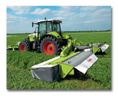
heavier during operation. The heavy-duty cutter bar is protected with Safety Link, which protects the cutterbar from internal damage when the cutterbar comes in contact with any external objects.
