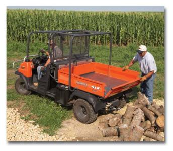
ing, towing of farm tractors/implements, removal of snow/manure, hauling of feed and materials, etc. The vehicle also features a newly modified variable hydrostatic transmission (VHT Plus) that delivers easier gear shifting and smoother transmission-assisted deceleration, as well as the new 24.8 hp Kubota diesel engine that provides 15 percent more horsepower than previous-generation RTV900s.
