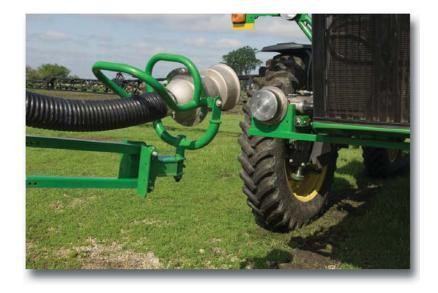
are joined and then inflates an air seal, locking the couplers. A plunger on the sprayer coupler actuates into the spring-return plunger on the tender vehicle, opening the passageway as the on-board pump begins loading. When the system detects that the tank is full, the pump shuts down, the plunger closes, the couplers unlock, and the arm disconnects as the operator drives away. Load Command<sup>TM</sup> can fill the 4,542.5 L (1,200 gal) tank as fast as three minutes.
