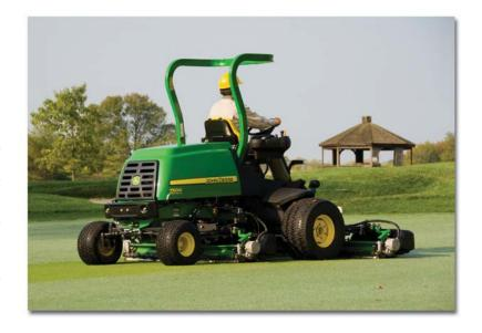
leak points, the E-Cut<sup>TM</sup> Hybrid Fairway Mower can be operated at a reduced engine speed for noise reduction, as well as fuel savings up to 30 percent as compared to hydraulic units, and still maintain the same cut quality from start to finish.
