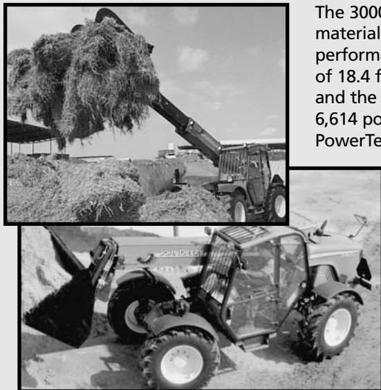
The 3000 Series Telehandlers from John Deere are rugged, purpose-built material handlers, designed to offer agricultural customers new levels of performance, lift capacity and maneuverability. The 3200 has a lift height of 18.4 feet (5.6 meters) and a capacity of 6,173 pounds (2,800 kilograms) and the 3400 offers a lift height of 23 feet (7 meters) and a lift capacity of 6,614 pounds (3,000 kilograms). Powered by the John Deere 4045
