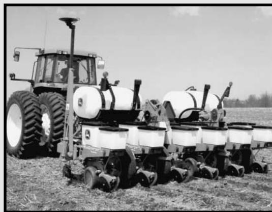
The machines plant in all field conditions such as conventional till, mulch till and true no till. They are equipped with MaxEmerge® Plus row units, which provide high strength, depth control and seed spacing. A new mounting bracket which allows the use of John Deere frame-mounted fertilizer openers is also available.
