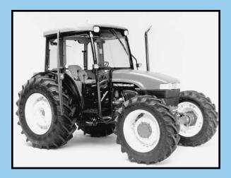
The New Holland Model TND and TNS Tractors are a line of compact, powerful, all-purpose utility tractors. TND models have a deluxe, fully suspended, fully enclosed cab in either 2WD or 4WD configurations. TNS models are available in deluxe or standard models. The six models in the series — TN55D, TN55S, TN65D, TN65S, TN75D and TN75S — produce up to 36 percent torque rise and run at low-rated speed of 2,300 rpm with three-cylinder displacement engines.
