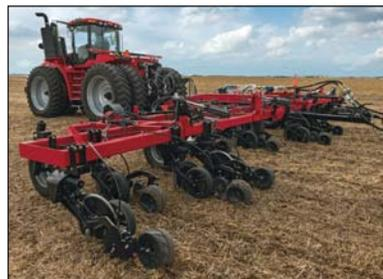
stability needed for high-speed operation, while the stubble-resistant radial tires prevent costly downtime due to tire failures and reduce soil compaction.
