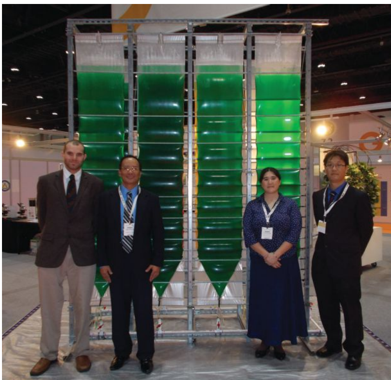
Cuello and his team at the University of Arizona designed a suite of photobioreactors that have improved liquid mixing and light incidence while using low-cost plastic materials, resulting in the proprietary zigzag or wave design of the Accordion PBR. Co-Inventors (left to right): Cody Lee Brown, Master’s candidate; author Cuello; Sara Kuwahara and Takanori Hoshino, postdoctoral researchers.
